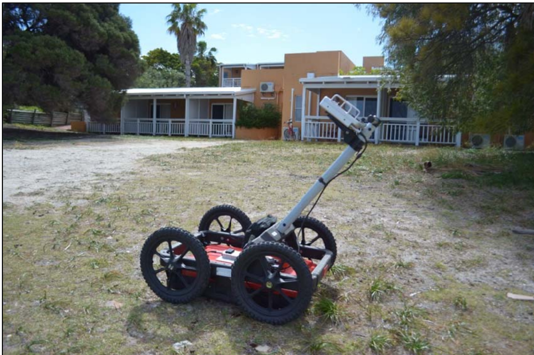
Plate 1: SWISS_RIA_2019_2019_03 Rottnest Lodge GPR Assessment – MALA Easylocator Pro Widerange RADAR
