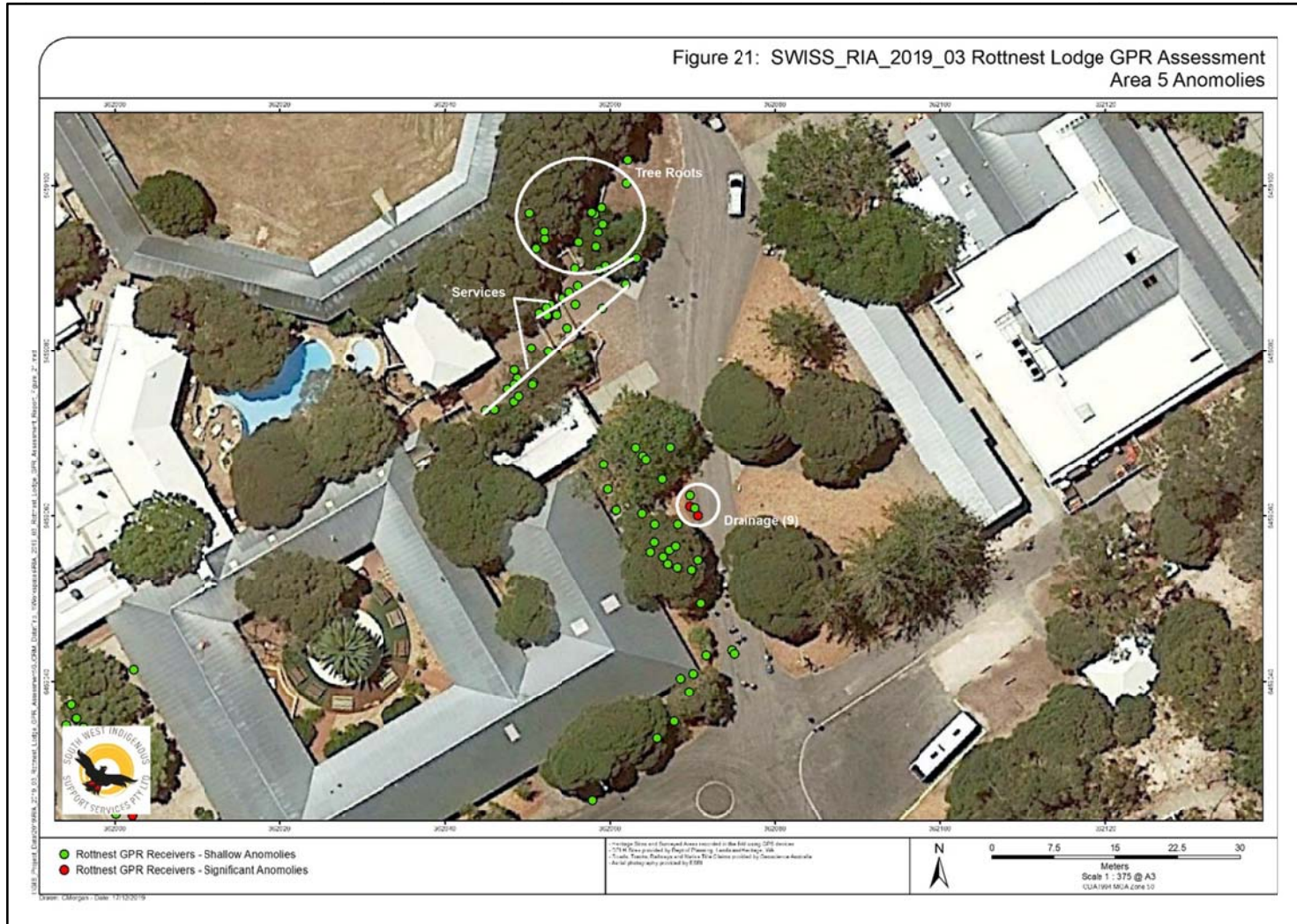
Figure 21: SWISS_RIA_2019_2019_03 Rottnest Lodge GPR Assessment – Area 5, Showing Interpreted Anomalies. Green circles indicate shallow anomalies and red circles indicate significant anomalies between 1 m and 2 m
