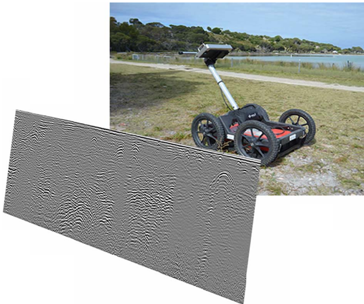
Figure 1: SWISS_RIA_2019_2019_03 Rottnest Lodge GPR Assessment – GPR and resultant radiogram
