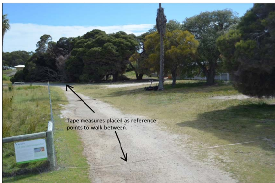
Plate 2: SWISS_RIA_2019_2019_03 Rottnest Lodge GPR Assessment – Garden Lake showing tape measures for line spacing control
