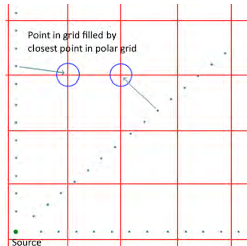
Figure B-2. Example Cartesian Grid Calculation
