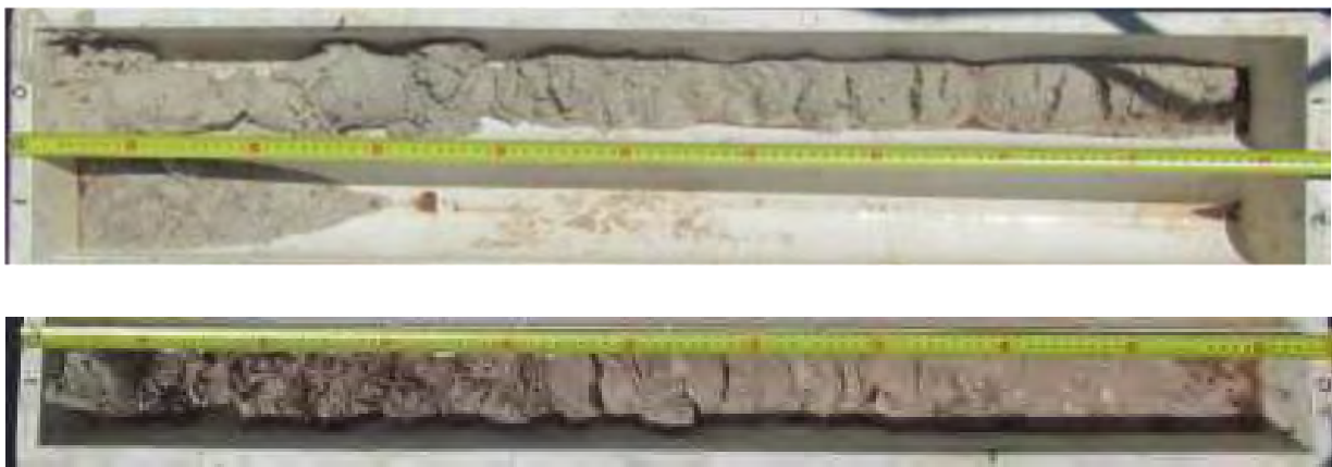
Figure 3.5: Core Samples for sample 2 (top) and sample 27 (bottom) (Douglas Partners, 2019). Cores are collected to the target depth below seabed of 1m, and demonstrate very low fines content and non-cohesive nature of the sediments at these locations
