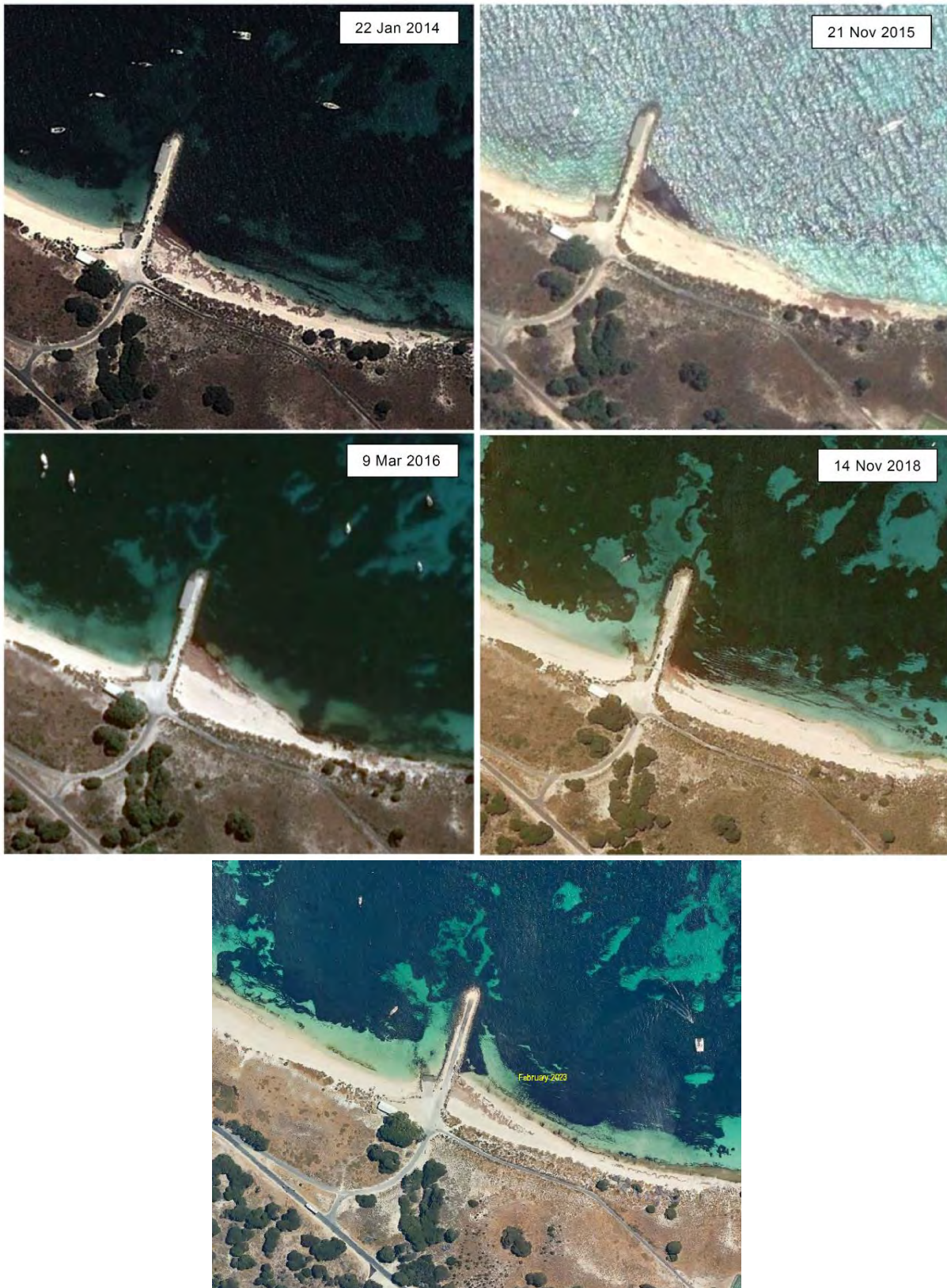
Figure 5.3: Aerial photography indicating the buildup of seagrass wrack between 2014 and 2023, largely on the eastern side of the Army Groyne (adapted from MRA 2019)
