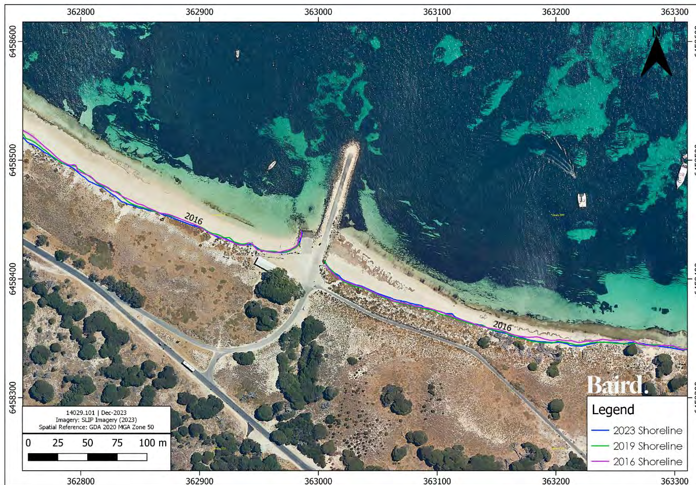
Figure 4.16: Overview of the latest shoreline movements, showing the 2019 and 2023 shorelines aligned to the 2016 shoreline
