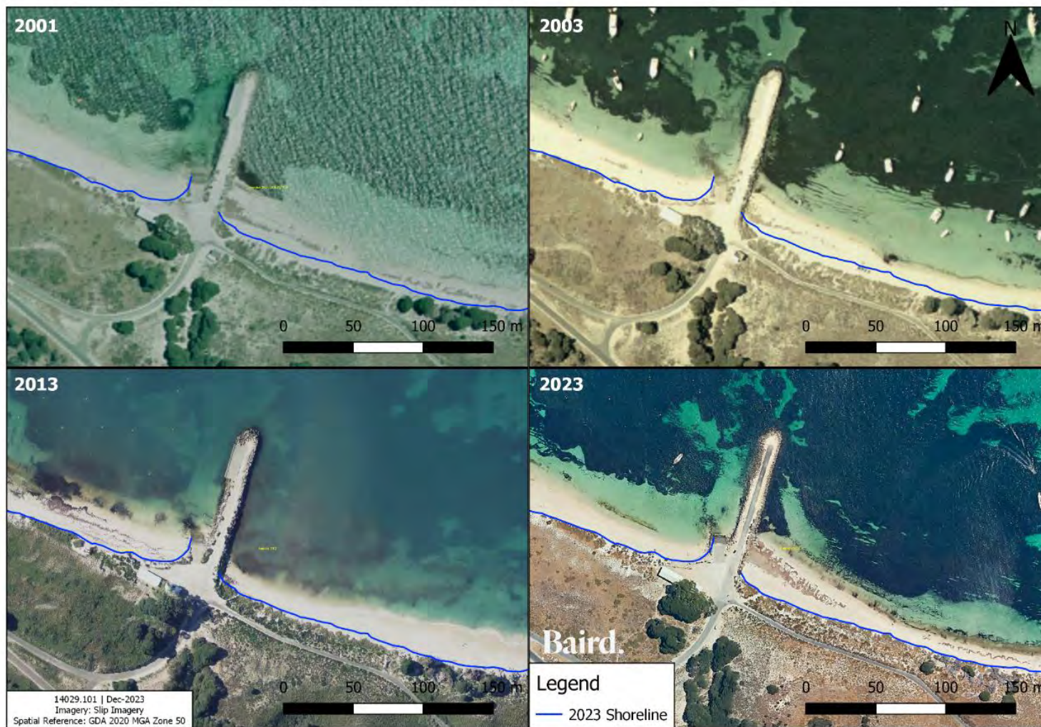
Figure 4.9: Historical aerial images from 2001 to 2023 adjacent the Army Groyne overlaid with the 2023 shoreline (proxied by the 2023 vegetation line)
