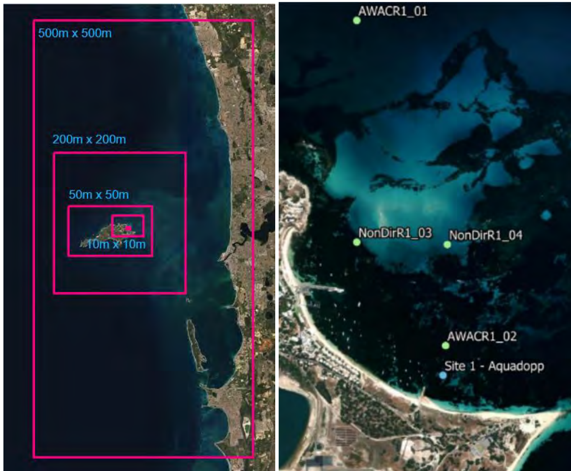
Figure 3.1: Left: Model domain for the hindcast SWAN wave model (Baird (2021)). Right: Thomson Bay measured data locations for the calibration.
