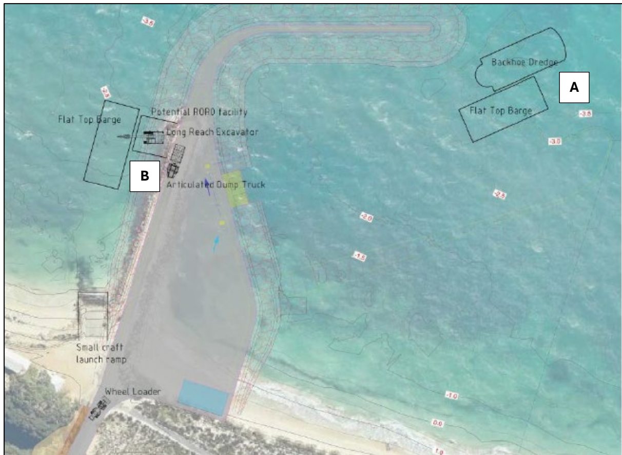
Figure 1: Indicative location of dredging equipment and barge for loading of dredge spoil (A), and location of barge and excavator on RORO facility for unloading dredge spoil into a ATD (B).
