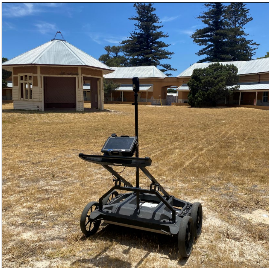
Figure 4: StreamDP GPR data acquisition using the StreamDP within the Quod (Area-01).
